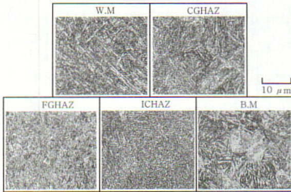
Fig. 2 Microstructures of virgin weldment
