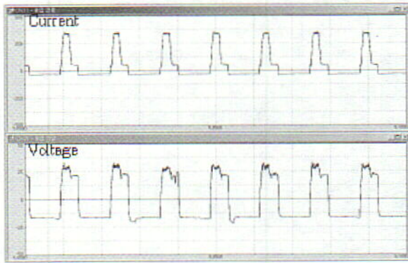
Fig. 12 Waveform at EN ratio 40% in polarity control AC pulse MIG welding(Current 60A)
