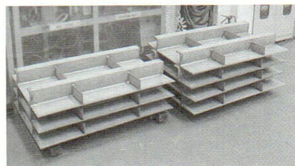
Fig. 12 Specimens of welded stiffened plates
