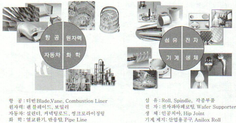
Fig. 2 Application field of thermal spray coating technology
