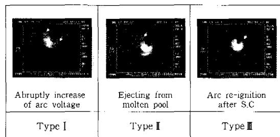
Fig. 11 Classification of spattering phenomena in short circuit transfer region of  $\text{CO}_2$  welding
