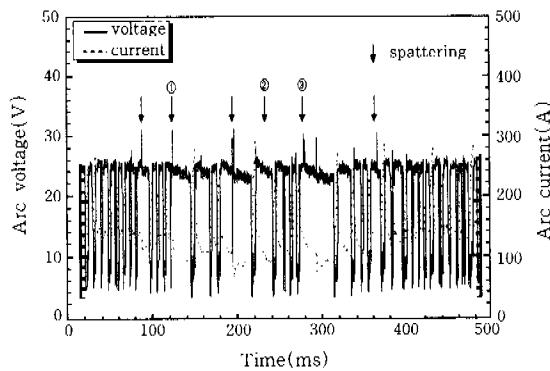
Fig. 7 Spatter generation of SM wire in short circuit transfer region
