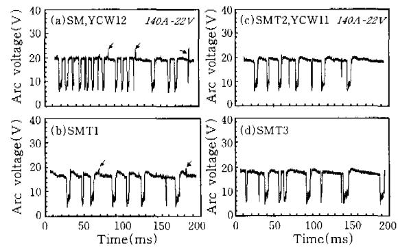
Fig. 3 Behavior of arc voltage in the region of short circuit transfer
