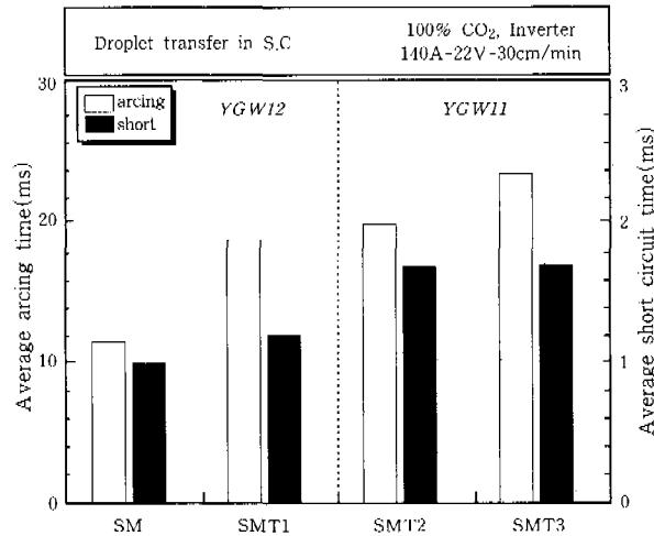
Fig. 4 Effect of wires on arcing time and short circuit time
