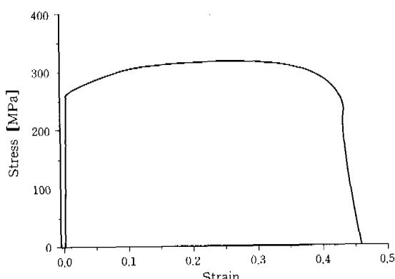
Fig. 1 Result of tensile test for case specimen
