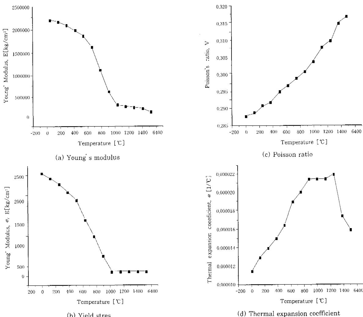
Fig. 6 Mechanical properties with temperature
