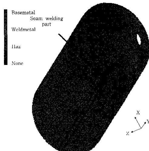
Fig. 5 Mesh generation considering seam weldment of case
