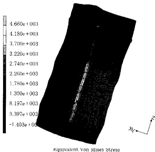
Fig. 7 Result of analysis considering initial shape and weldment of case
