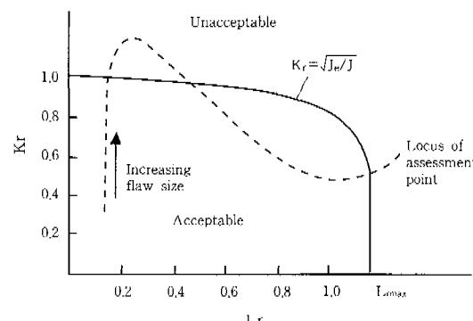
Fig. 6 High level FAD (level 4 in Table 1) established thorough the elastic-plastic fracture mechanical analysis<sup>9)</sup>
