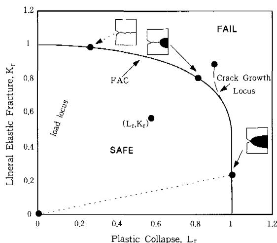
Fig. 1 Typical failure assessment diagram (FAD)<sup>12)</sup>
