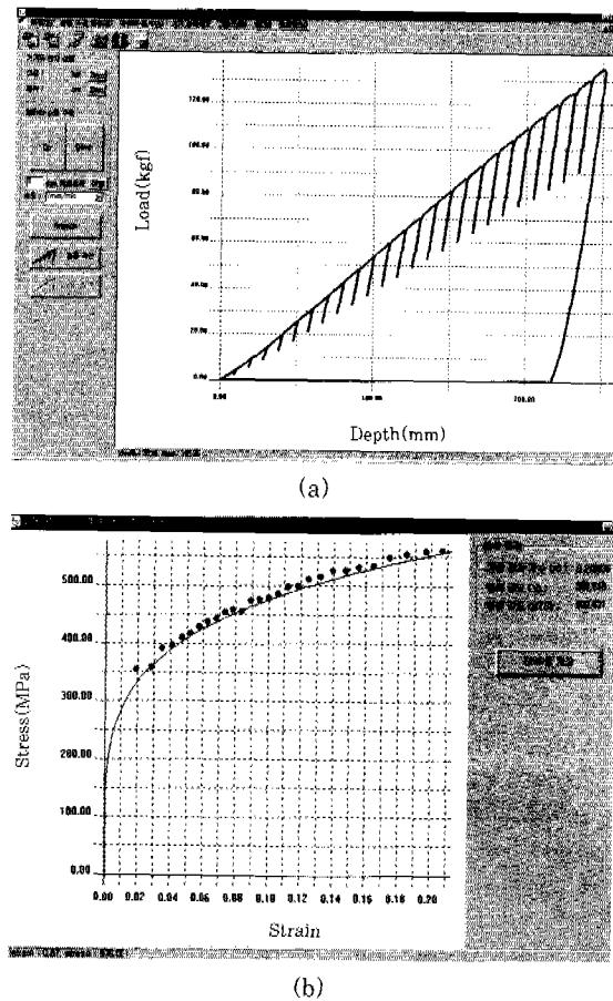
Fig. 10 Examples showing the results from continuous indentation test: (a) indentation load-depth curve and (b) tensile flow curve obtained from (a)
