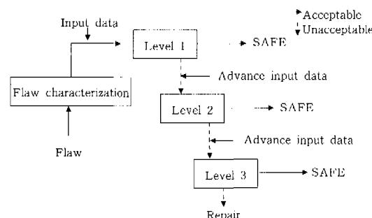
Fig. 5 General procedure of flaw assessment using FAD
