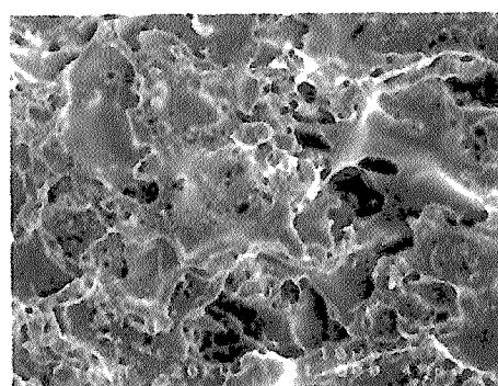
Photo 1 SEM surface morphology of plasma sprayed WC-12%Co coating
