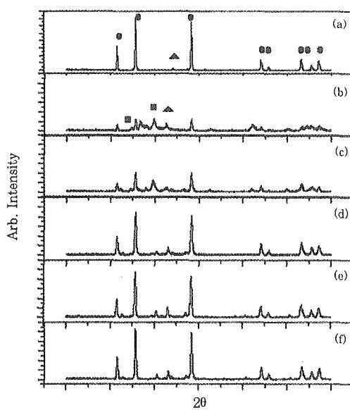
Fig. 1 X-ray diffraction patterns of plasma sprayed WC-Co coatings at various heat treatment temperature. (● : WC, ■ :  $\text{W}_2\text{C}$ , ▲ :  $\text{Co}_3\text{W}_3\text{C}$ )
