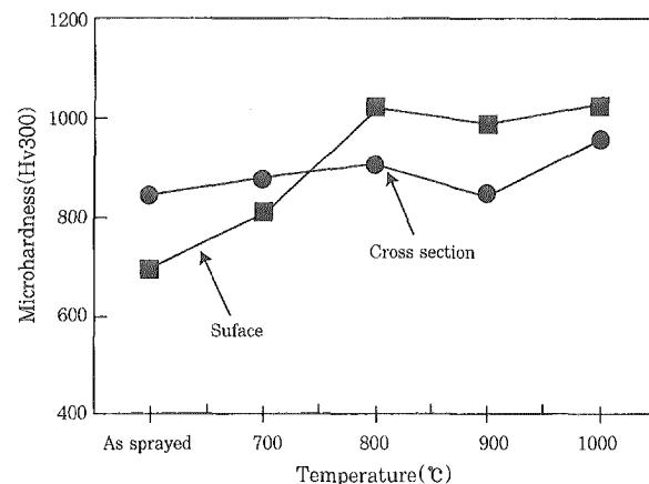
Fig. 2 Relationship between microhardness and heat treatment temperature.
