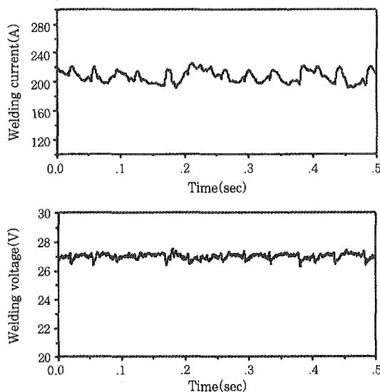
Fig. 5 Experimental current and voltage waveforms in globular mode
