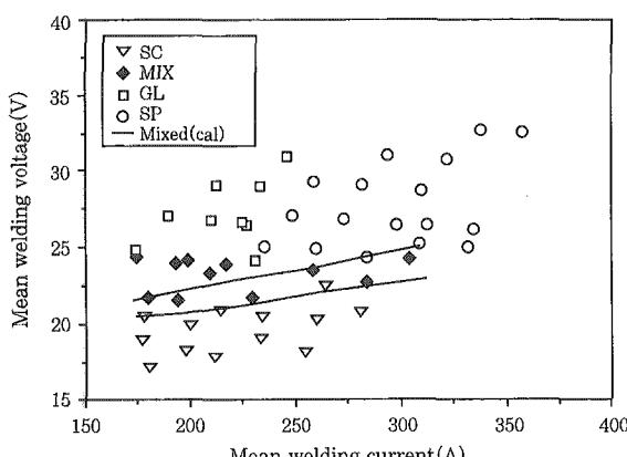
Fig. 12 Comparison of experimental and predicted metal transfer modes
