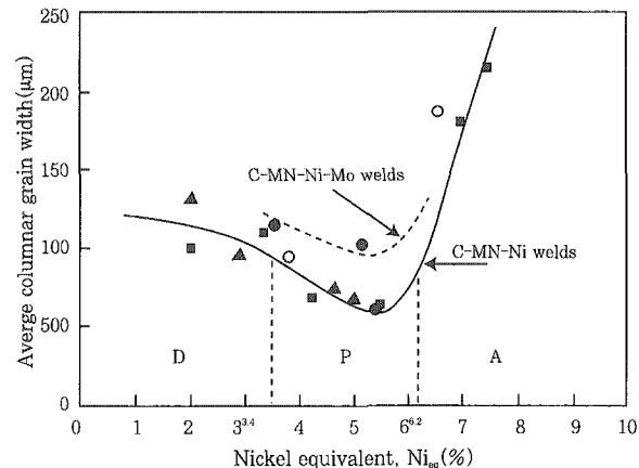
Fig. 4 Influence of nickel equivalent on the columnar grain size<sup>4)</sup>
