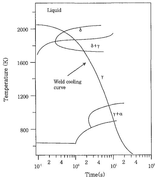
Fig. 1 Schematic diagram of continuous cooling transformation diagram
