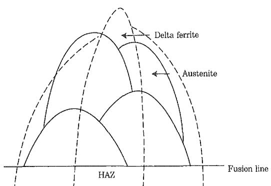
Fig. 2 Schematic illustration of austenite grains nucleating from primary delta ferrite grain boundaries<sup>1)</sup>.
