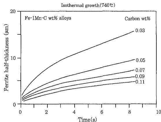
Fig. 6 An illustration of parabolic thickening of grain boundary ferrite during isothermal transformation<sup>17)</sup>
