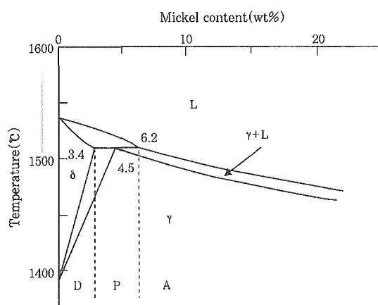
Fig. 3 Fe-Ni equilibrium phase diagram (high temperature section) (D : primary  $\delta$ -ferrite solidification, P: peritectic effect, A: primary austenite solidification)
