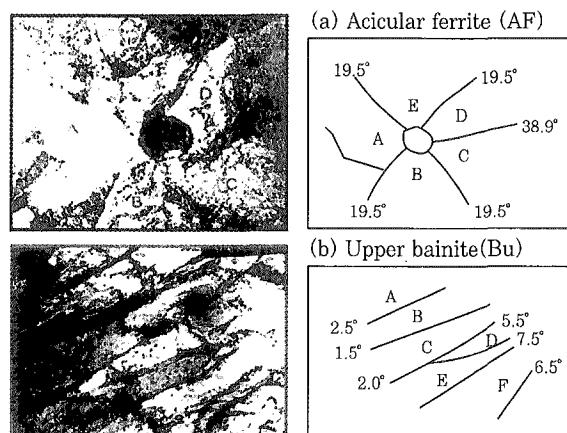
Fig. 10 Misorientation angle of lath structures : (a) acicular ferrite and (b) upper bainite<sup>24)</sup>.
