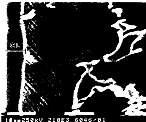
Fig 2 SEM micrograph showing compound layer(CL) by plasma nitriding of Stellite
