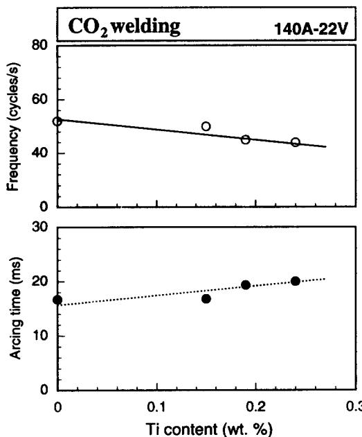
Fig. 3 Effect of Ti content on droplet transfer in low current range
