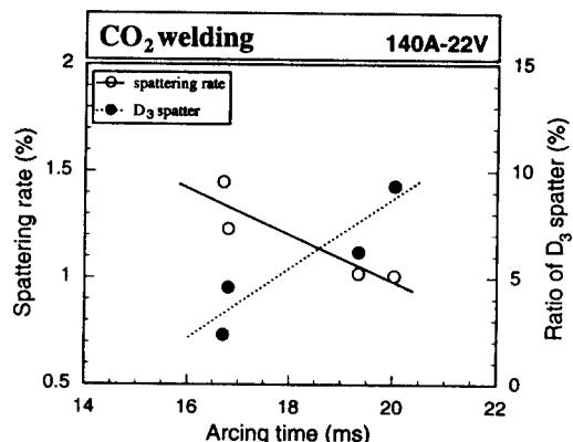
Fig. 7 Effect of arcing time on spatter generation
