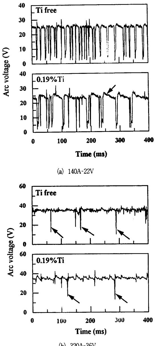
Fig.2 Effect of Ti content on arc voltage change
