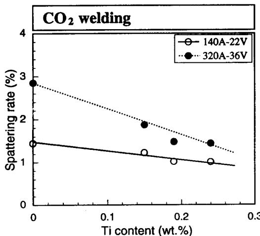
Fig. 5 Effect of Ti content on spattering rate
