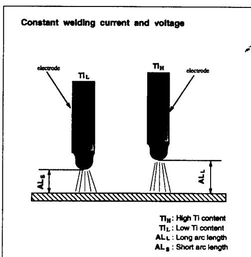
Fig. 8 Schematic diagram for effect of Ti on arc phenomena
