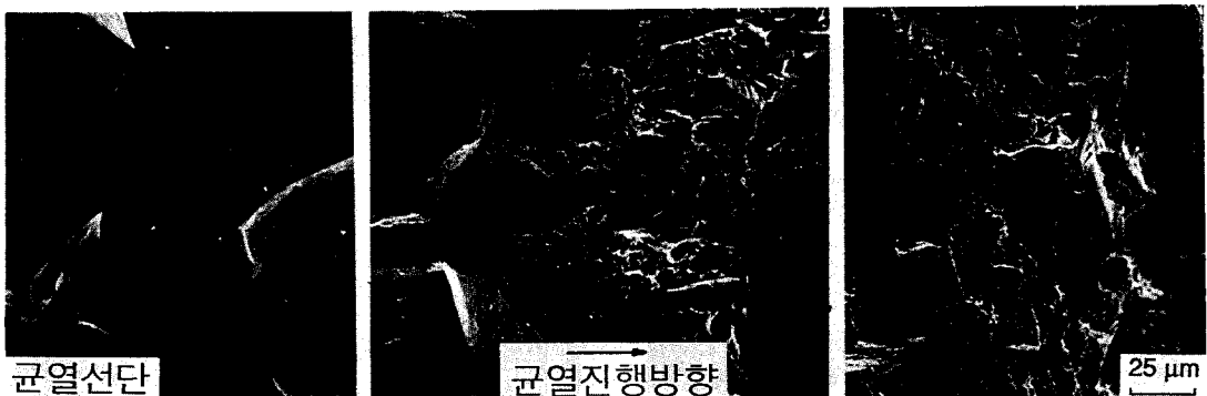
Fig 11. Transition of reheat crack of the heat affected zone ffrom 1150°C single cycled
