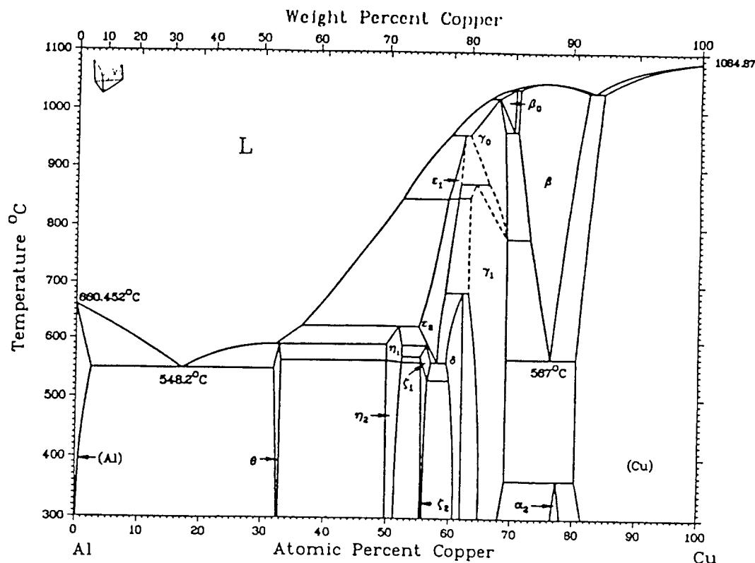
Fig. 1 Binary alloy phase diagram of Al/Cu<sup>7)</sup>
