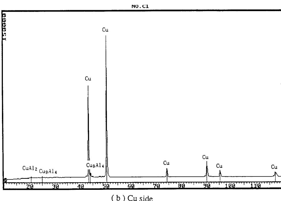
**Fig. 3** Results of X-ray analysis at fractured surface for Al/Cu(C-1)
