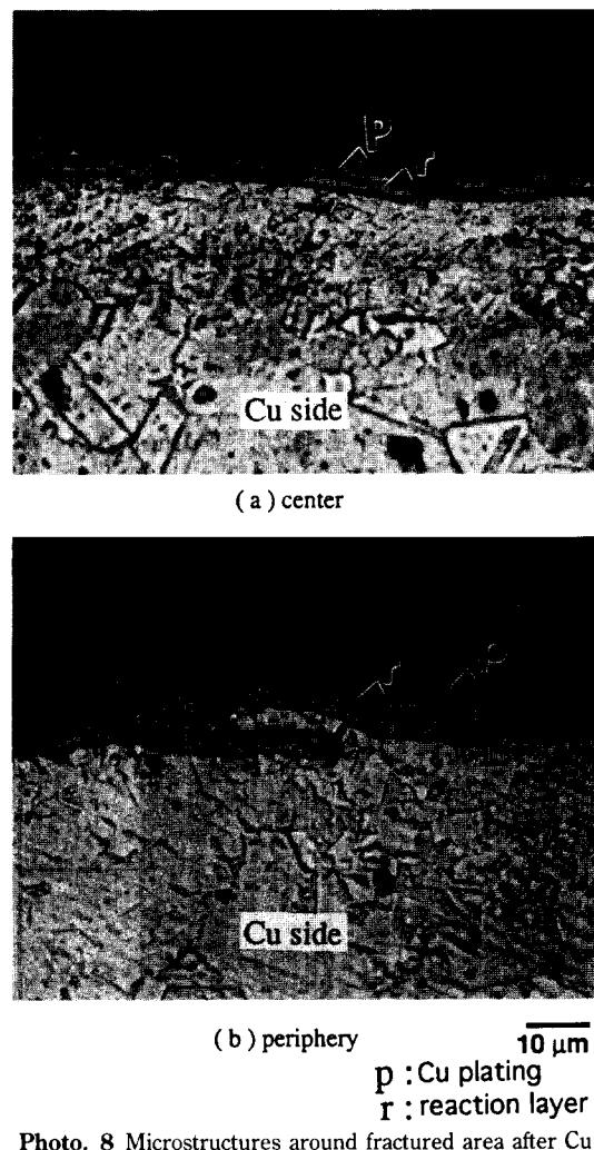
Photo. 8 Microstructures around fractured area after Cu plating on Cu side(C-5)
