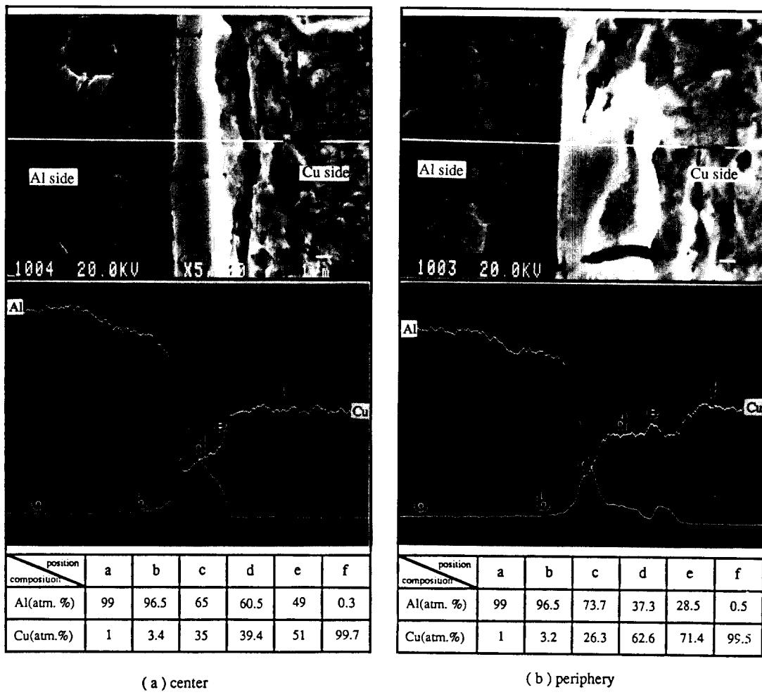
Photo. 4 EDAX analysis along arrow direction of Al/Cu joint (C-5)
