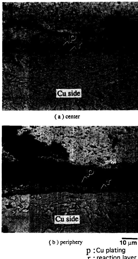
Photo. 7 Microstructures around fractured area after Cu plating on Cu side(C-1)
