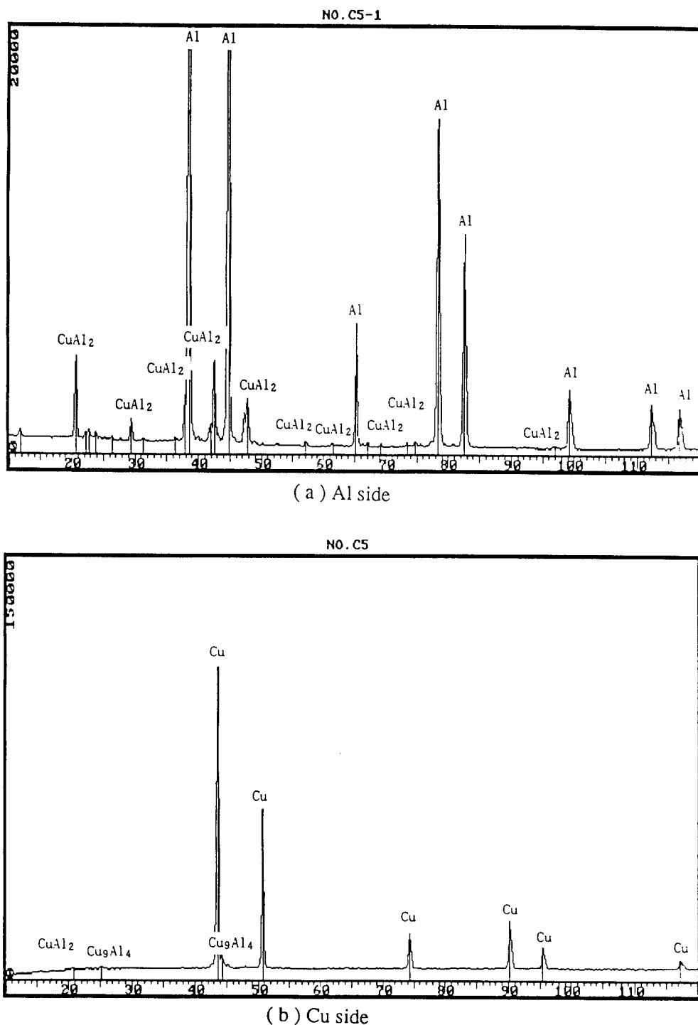
Fig. 4 Results of X-ray analysis at fractured surface for Al/Cu(C-5)
