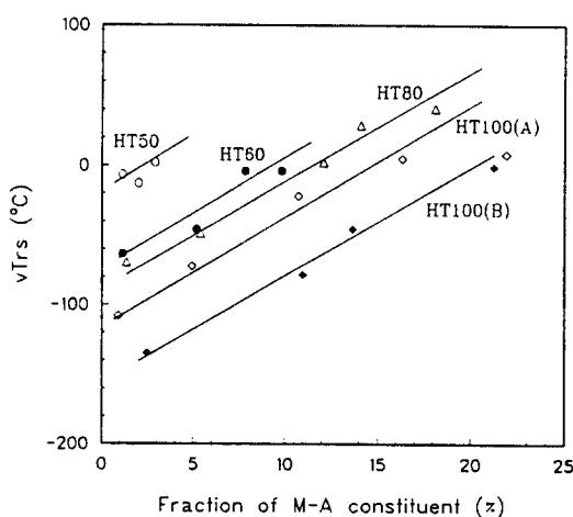
Fig. 5 Variation of HAZ Toughness with Fraction of M-A Constituent<sup>3)</sup>.
