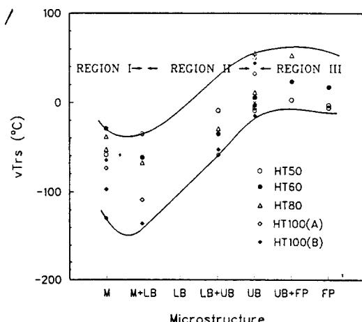
Fig. 3 Relationship between Microstructure and HAZ Toughness<sup>3</sup>.
