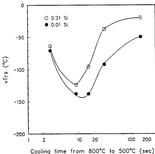
Fig. 8 Effect of Lowering Si Content on the HAZ Toughness in HT80 Steel<sup>14</sup>.
