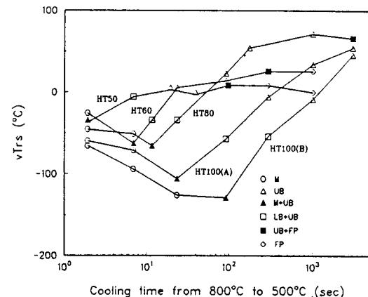
Fig. 2 Variation of HAZ Toughness with Cooling Time from  $800^\circ\text{C}$  to  $500^\circ\text{C}$ <sup>3</sup>.
