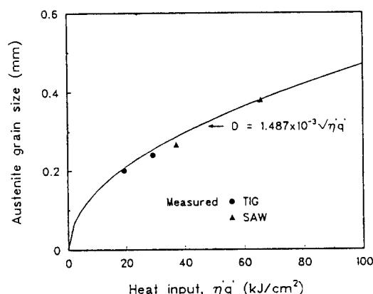
Fig. 1 Variation of Austenite Grain Size with Heat Input in HT80 Steel<sup>2</sup>.
