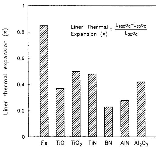
Fig. 7 Liner Thermal Expansion Behavior (from 20 to 600°C) of Several Compounds<sup>6,7</sup>.
