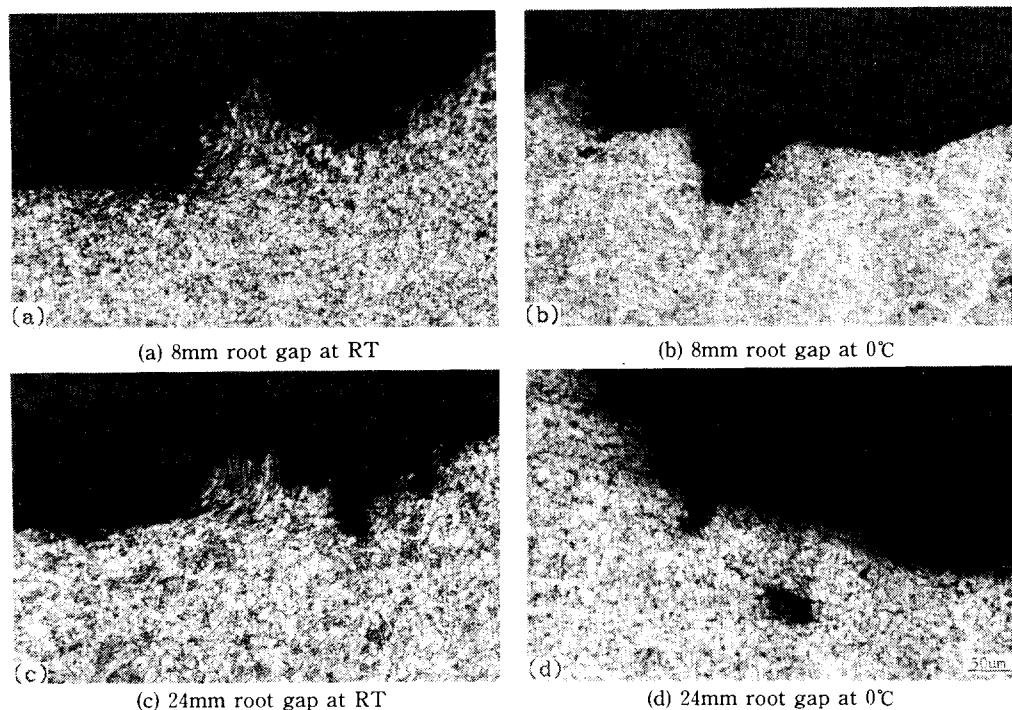
Fig. 16 Microstructures of lateral surfaces near cracked regions
