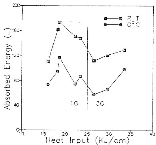
Fig. 9 Variation of absorbed energy with heat inputs
