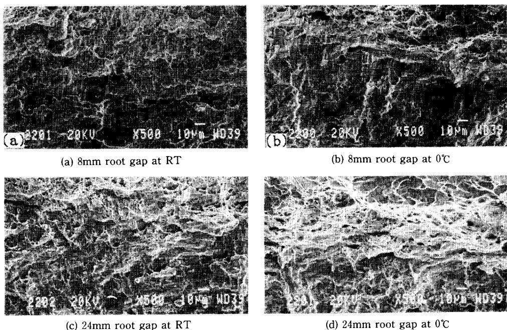
Fig. 15 S.E.M observation of fractured surfaces after CTOD test at RT and 0°C
