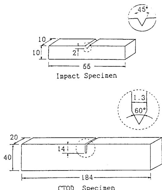
Fig. 2 Configuration of CTOD and impact test specimens
