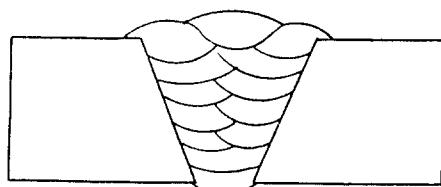
Fig. 1 Weld joint design and weld metal deposit
