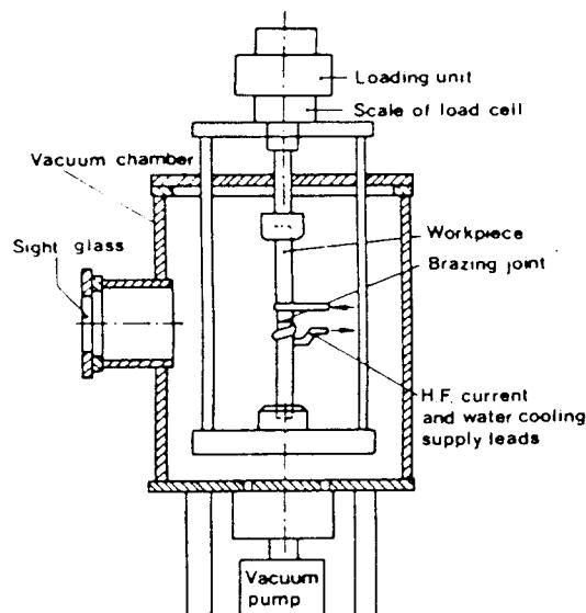
Fig. 2 Schematic diagram of high frequency induction furnace
