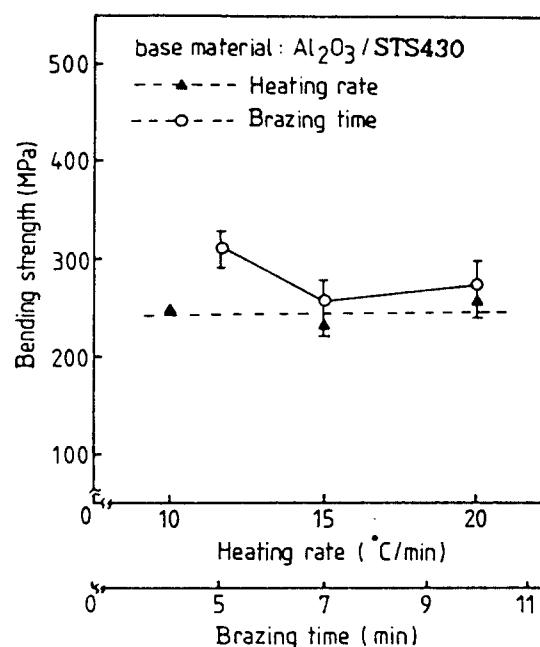
Fig. 10 Bending strength of brazed  $\text{Al}_2\text{O}_3/\text{STS}430$  joints with different brazing conditions
