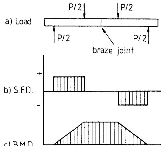
Fig. 4 S.F.D and B.M.D. in 4-point bending test
