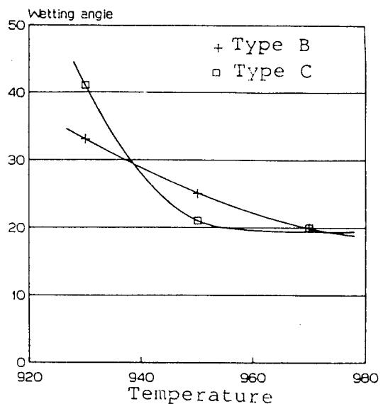
Fig. 5 Results of wettability test on  $\text{Al}_2\text{O}_3$
