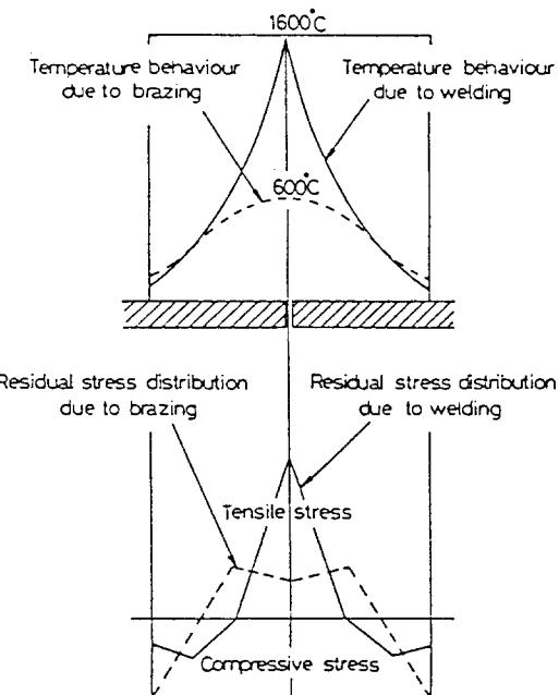
**Fig. 1** Comparision of heat affected zones produced by welding and brazing
