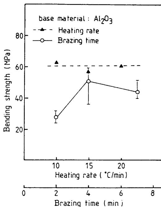
Fig. 8 Bending strength of brazed  $\text{Al}_2\text{O}_3/\text{Al}_2\text{O}_3$  joints with different brazing conditions.
