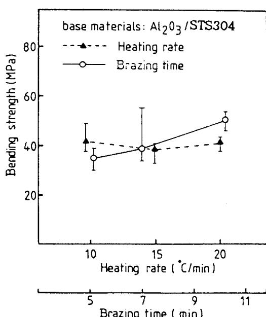
Fig. 9 Bending strength of brazed  $\text{Al}_2\text{O}_3/\text{STS}304$  joints with different brazing conditions
