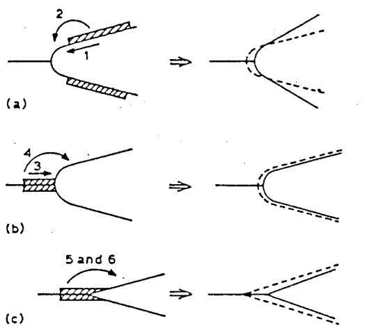
\* surface source mechanisms (1 and 2); b bond-line source mechanisms (3 and 4); c bulk deformation mechanisms (5 and 6)
