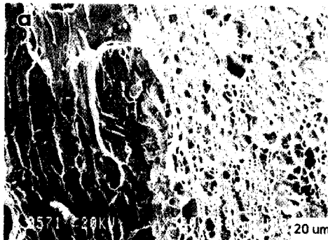
Photo 5. SEM fractographs of base metal impact specimen tested at -196^{\circ}\text{C} (a) and the magnified fractograph of ductile region in photo a (b), whereas notch tip is located at the upper part of each photo.
