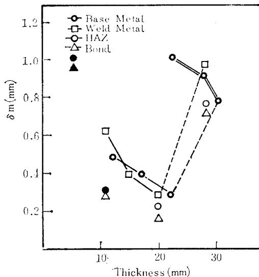
Fig. 7. Comparison of the critical COD( $\delta_m$ ) of each base metal with those of weldments.
