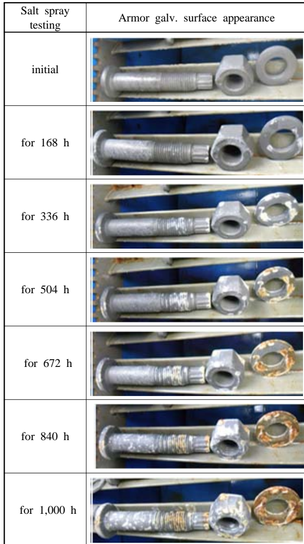
Fig. 6 Salt spray testing result of Armor Galv. specimen for 1,000 h
